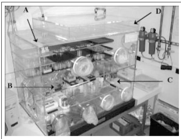
**Figure 1.** The environmental weighing and conditioning chamber. A: main chamber, B: sliding door, C: insertion/removal door, D: RH control chamber.
